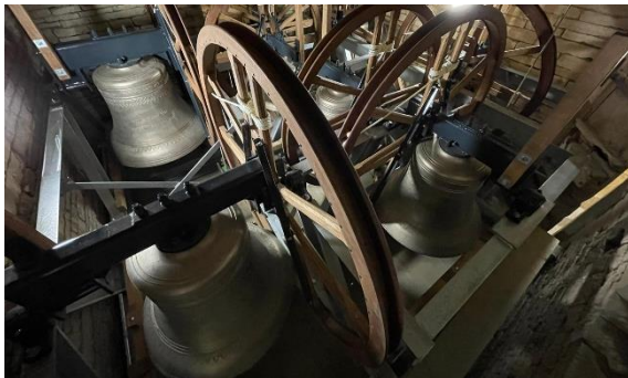
Figure 1. Bells “down” as the general public would always see them (the new Allanconi 8 at Hawkesbury, Glos. Courtesy M. Higby)
