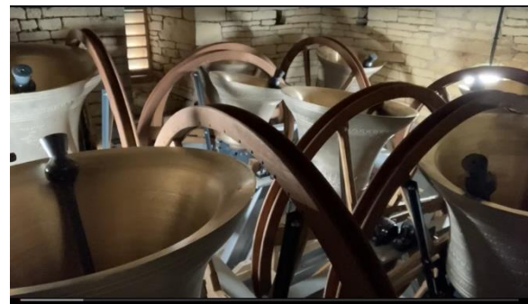
Figure 2. The same bells being rung “full circle”, so they spin nearly 360° on each revolution
